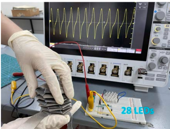
Fig. 15. Demonstration of using the fabricated Origami-inspired TENG to power 28 LEDs connected in series.
